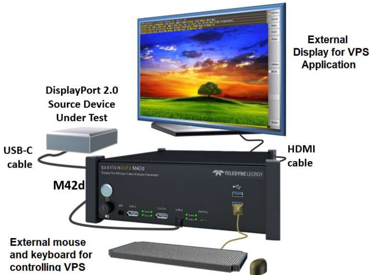
VPS GUI Running on External Display (Source Test Example)
